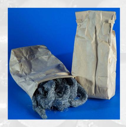
**Lead wool**, a form of caulking lead, consists of long, fine strands of chemical-grade lead twisted into 5/8" rope for use in various applications.
