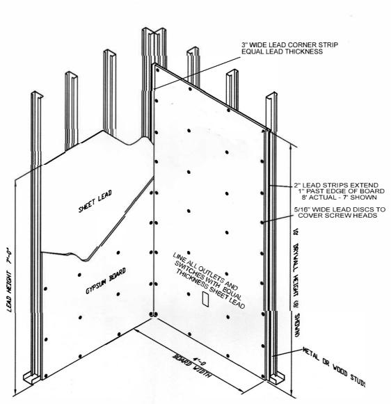
MAYCO lead-backed gypsum wallboard is furnished as 1/2" and 5/8" fire code gypsum board meeting classification ASTM C 1396 with pure lead sheet meeting federal specification QQ-L-201 F, which is factory laminated to the back side of the gypsum panel. The lead extends over the width of the gypsum board and 2" strips are included to cover the vertical joints between each of the boards. Strips are also required at the corners.
